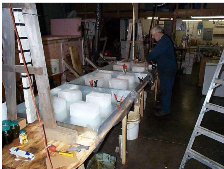
Figure 2. 1-m 2 pans used for preliminary screening tests.
