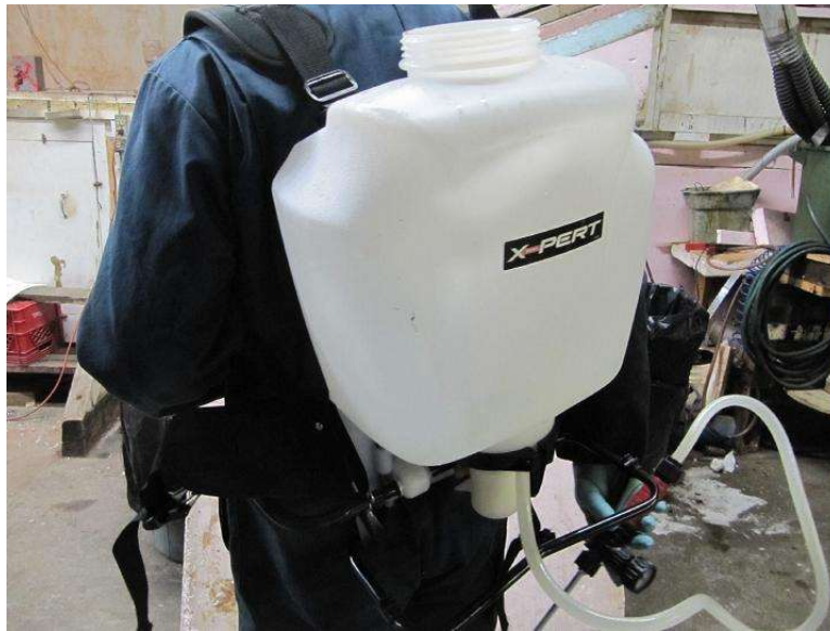
Figure 37. Commercial backpack sprayer recommended for small-boat application system.
