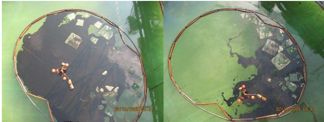
Figure 31. Overhead view of disc skimmer test with 10% ice before and after herding.
