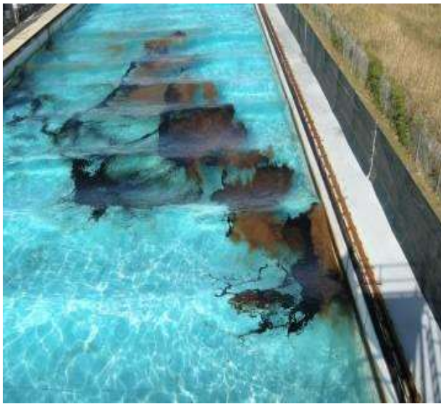
Figure 36. Oil beginning to disperse after treatment and waves on.
