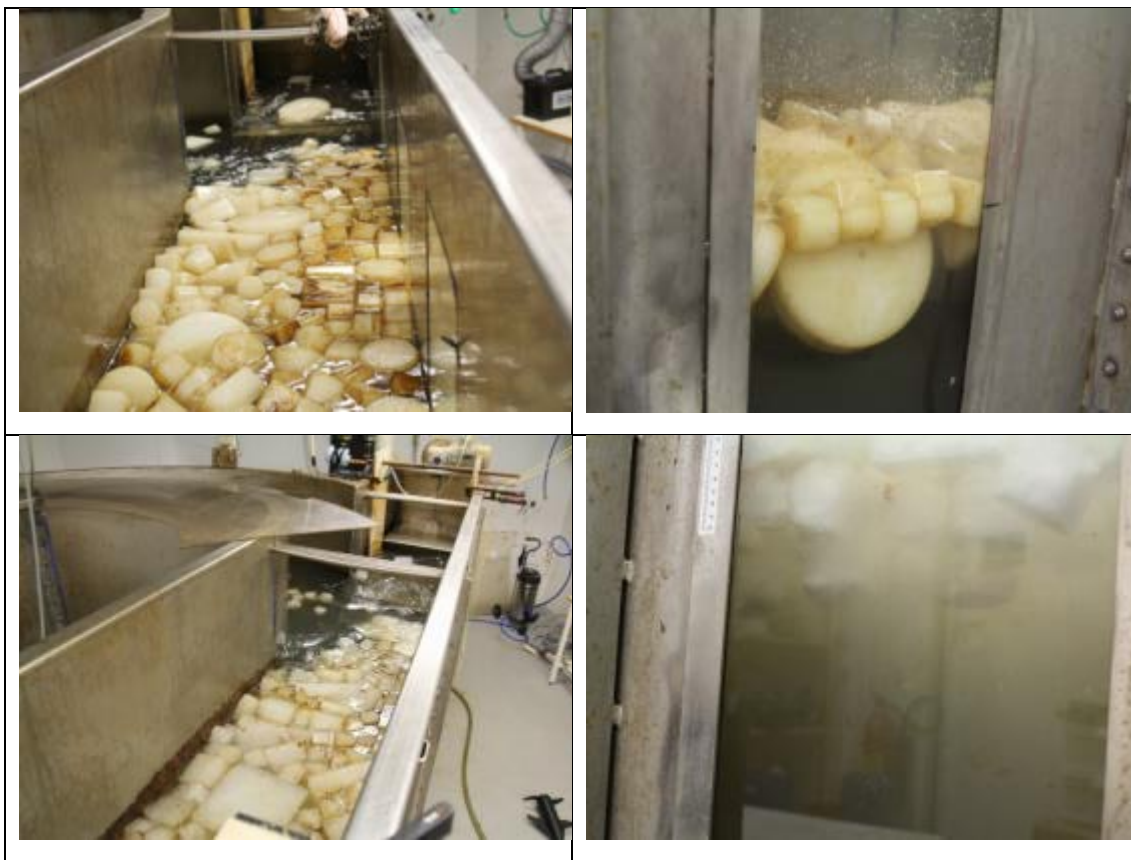
Figure 3.4 Test tank experiments at high energy: PE blocks in upper photos, and natural ice in the lower photos.
