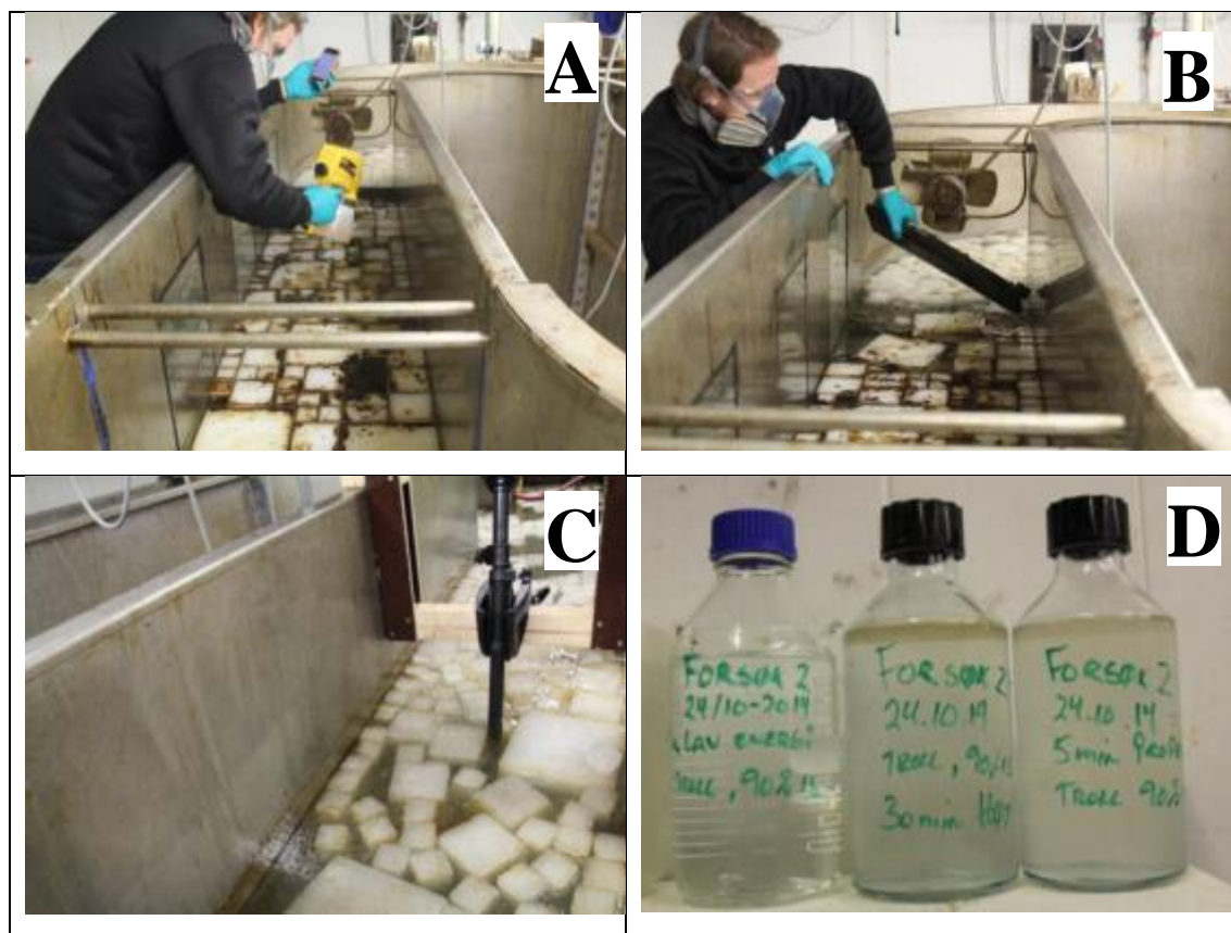
Figure 2.6 Dispersant application (A), removing barriers after 18 hours of oil weathering (B); Positioning of propeller (C); Water samples from experiment with natural ice (D).
