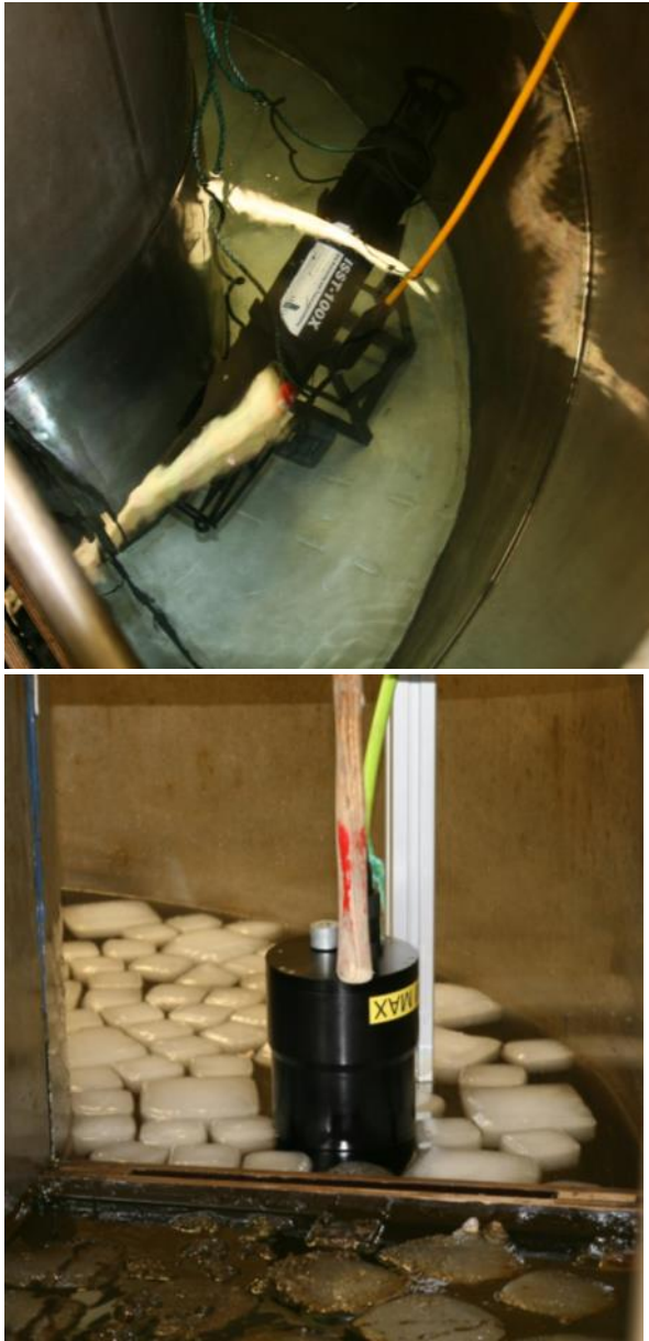
Figure 2.2 SINTEF flume prior to dispersion: LISST positioned horizontally at 50 cm depth (left) and SilCam positioned vertically with monitoring at 50 cm depth (right photo).
