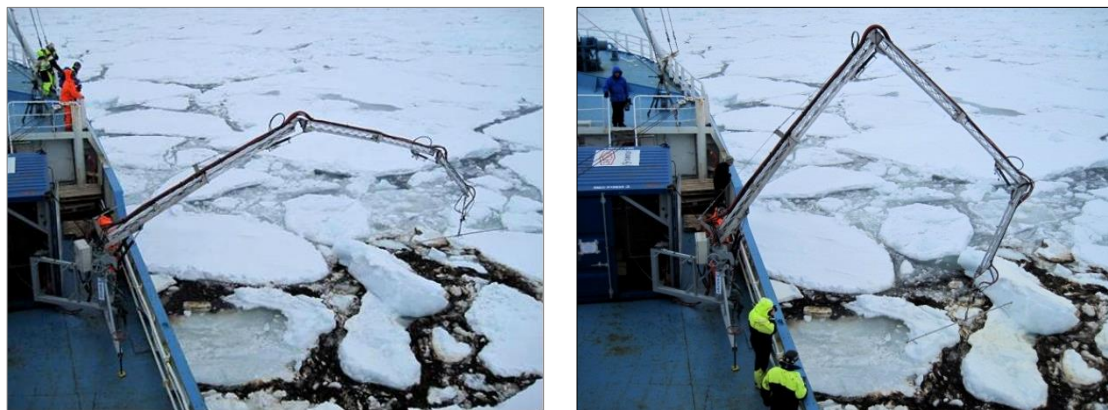
Figure 1. Prototype manoeuvrable spray system being used to spray dispersant onto oil in ice
