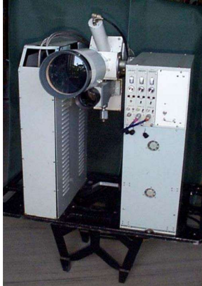
Figure 26. ATMARIL-3 on-board LIDAR. From the pamphlet of the Institute of Atmospheric Optics SB RAS, Russia, http://www.sbras.nsc.ru/dvlp/eng/pdf/059.pdf
