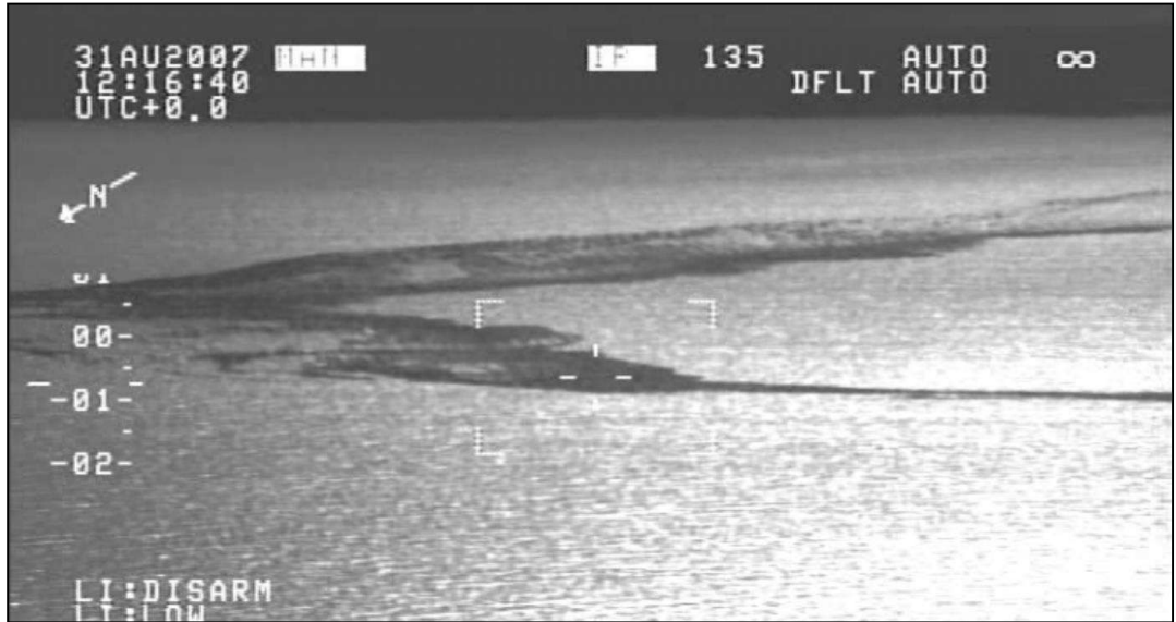
Figure 13. Example of FLIR image of oil spill (from Domargård, 2012).
