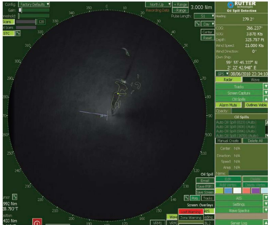
Figure 18: Vessel-based oil spill surveillance using Rutter Sigma S6 (from Safer, 2011)
