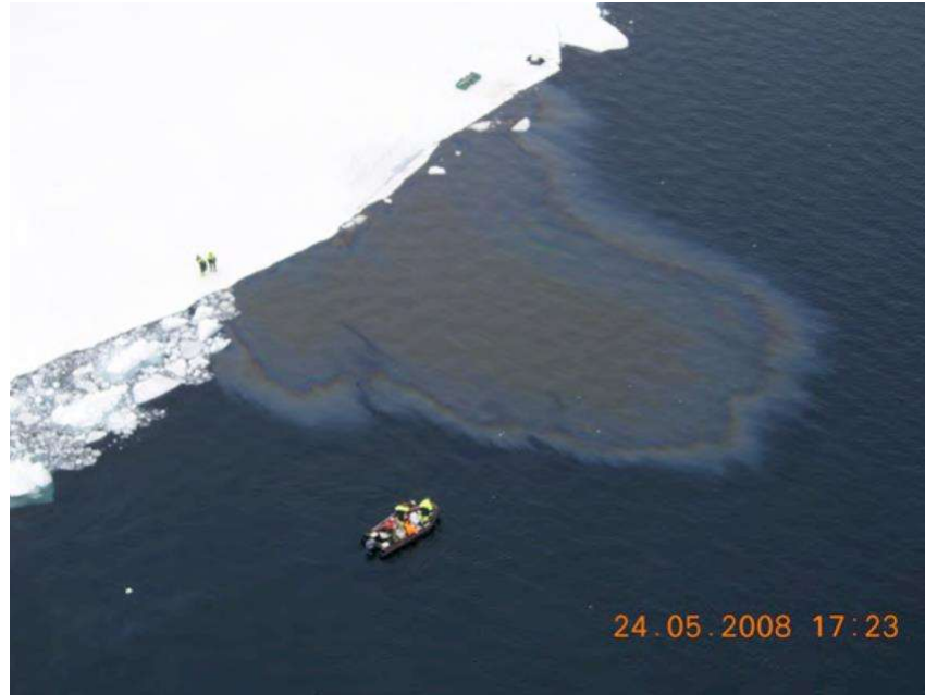
Figure 7. Aerial photograph showing oil being released into ice-affected water during the SINTEF JIP field experiments carried out in 2008 (from Dickins, 2010)
