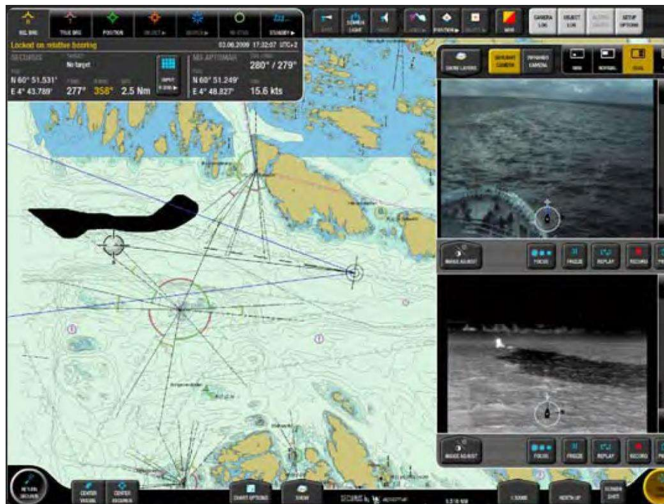
Figure 32. View of bridge console depicting spill location on ECS, digital video and TIR imagery
