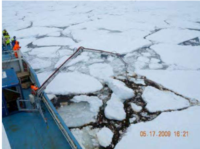
Figure 6. Photograph showing oil being released between ice floes during the SINTEF JIP field experiments carried out in 2009 (from Dickins, 2010)
