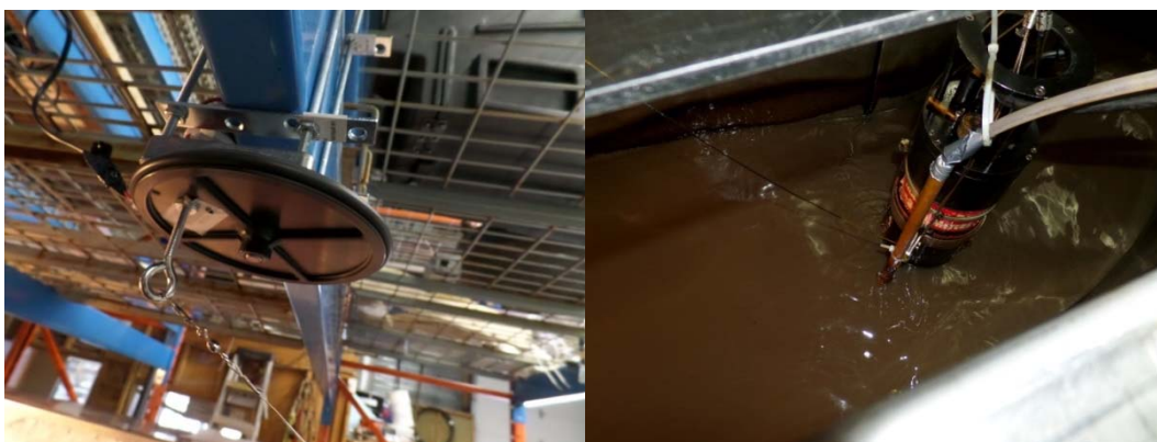
Figure 2. Motor, offset wheel and pull cord used to rock the Lisst particle size analyzer
