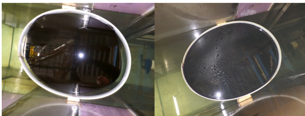
Figure 1. Oil in containment ring prior to and after dispersant application
