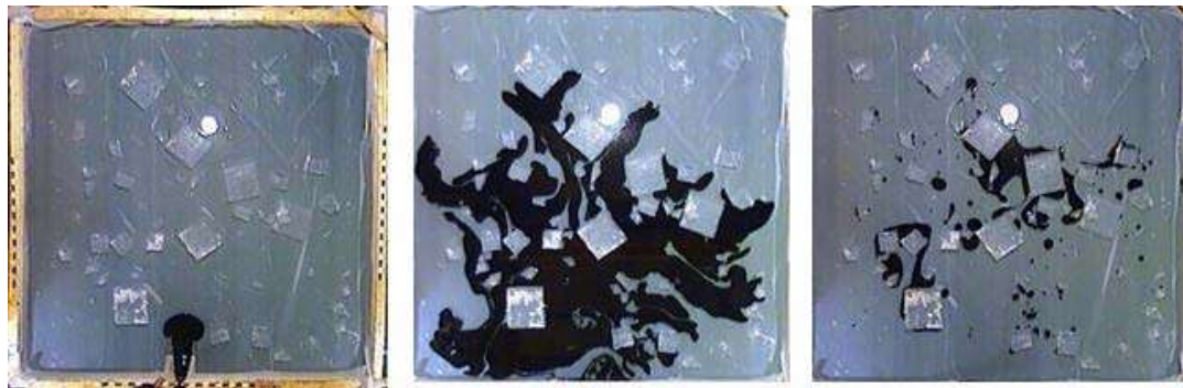
Figure 6-9 Testing of silicone-based herding agents at CRREL (far left shows oil release, Centre shows oil spread to equilibrium, Right shows contraction to new equilibrium after herder addition to water). (Source: SL Ross Environmental)
