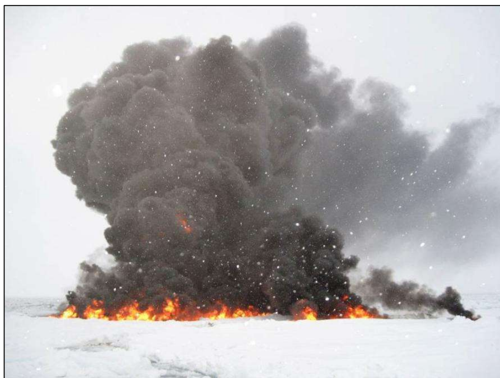
Figure 5-13 Burning 2 m 3 experimental spill in pack ice on the Barents Sea 2009. (Source: SINTEF)
