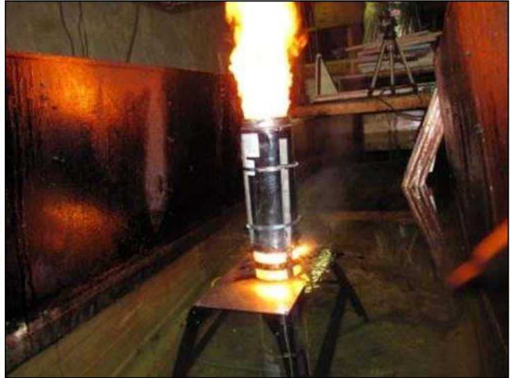
Figure 6-26 Small-scale floating burner test in an indoor wave tank. (Source: SL Ross Environmental Research)
