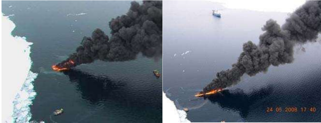
Figure 6-8 Burn of herded slick in Barents Sea pack ice lead (near start on left, near end on right). (Source: D. Dickins)
