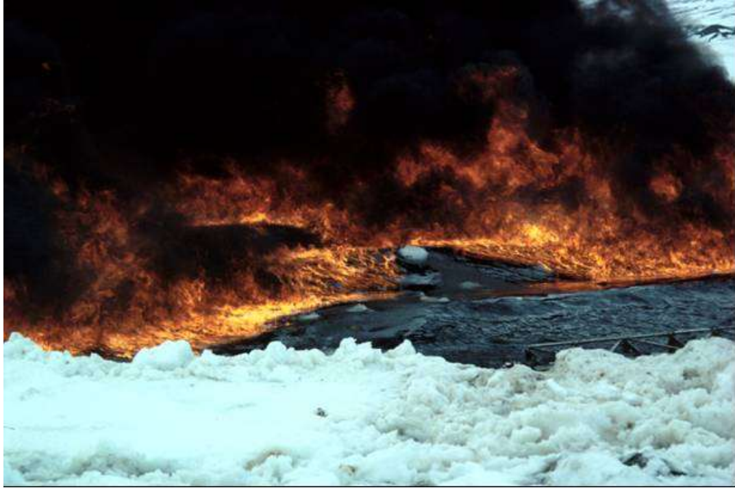
Figure 5-10 Burning oil in brash ice with waves at Svalbard 1992. (Source: I. Buist)
