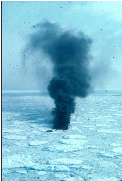
Figure 5-9 Burning crude oil in 9+/10ths pack ice off Cape Breton, 1986. (Source SL Ross Environmental Research)
