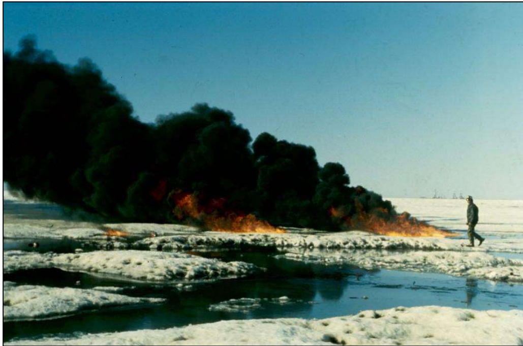
Figure 5-2 Burning crude oil from a subsea blowout under ice. (Source: I. Buist)
