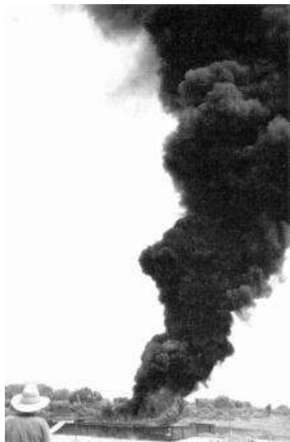
Figure 6-22 Burn test with no aeration. (Source: MSRC)
