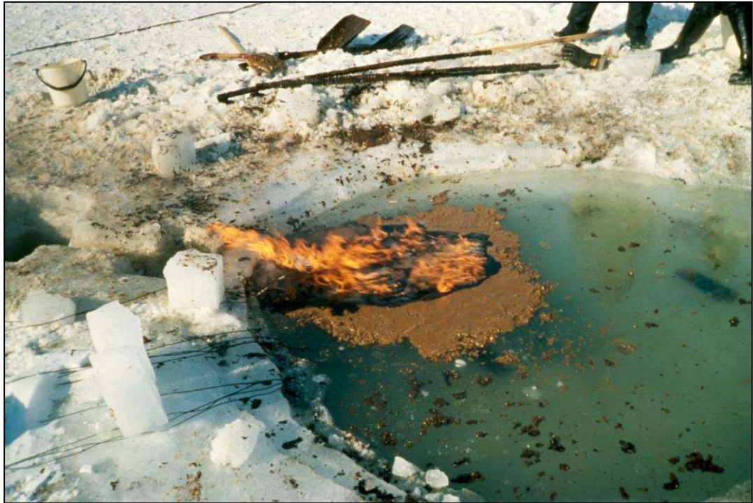
Figure 5-4 Igniting emulsions on water on ice with modified igniters. (Source: I. Buist)
