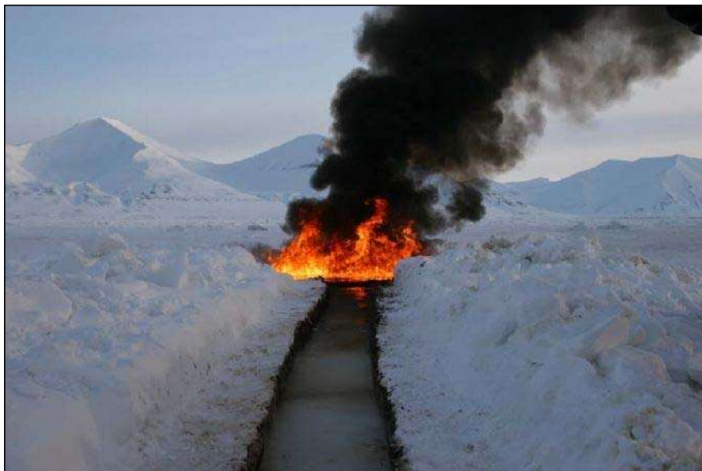
Figure 5-12 Burning oil weathered in brash ice in meso-scale burn pit at Svalbard, 2007. (Source: SINTEF)
