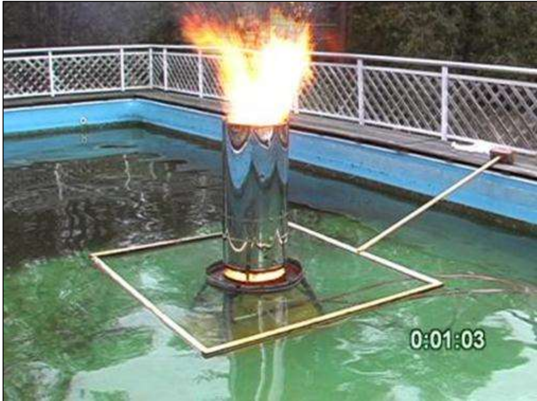
Figure 6-27 Mid-scale burner model during outdoor tests. (Source: SL Ross Environmental Research)
