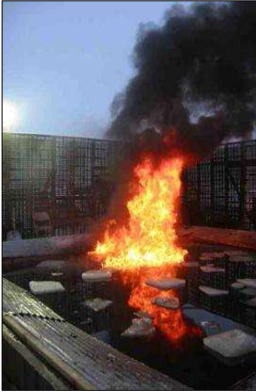
Figure 6-7 Burn test with ThickSlick 6535 at Prudhoe Bay, AK in 2006. (Source: J. Mullin)
