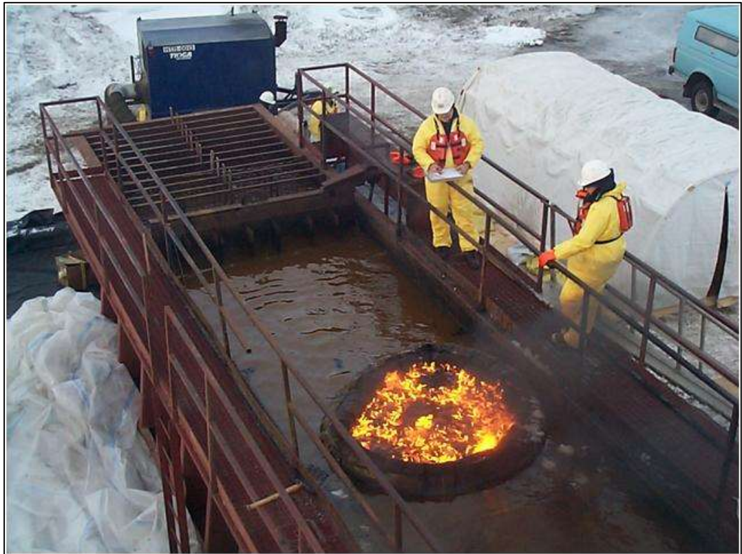
Figure 5-11 Test burns in brash ice with waves in Prudhoe Bay, 2003. (Source: D. Dickins)
