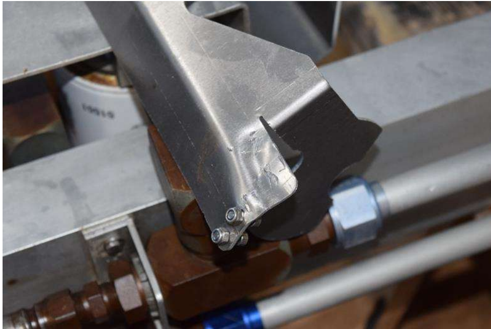
Figure 95. Damage to SIM from Jammed Cartridge
