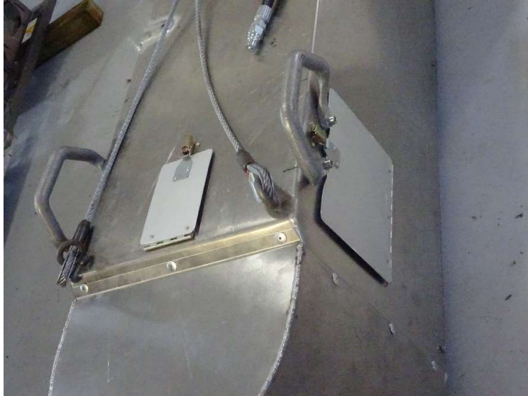
Figure 96. Access doors added to SIM
