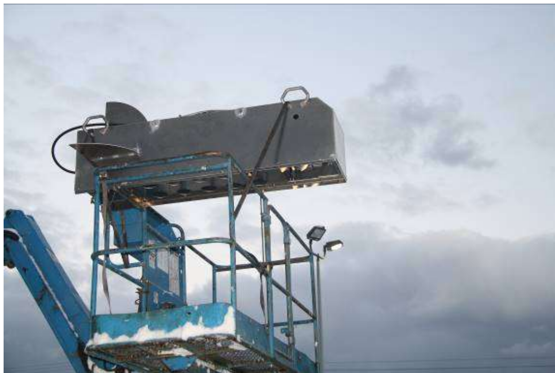
Figure 75 IIHAS strapped to person-lift basket and loaded with activated igniters
