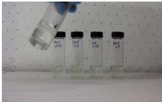
Figure 39. 15°C Diesel at 30 minutes with 0.10g gel
