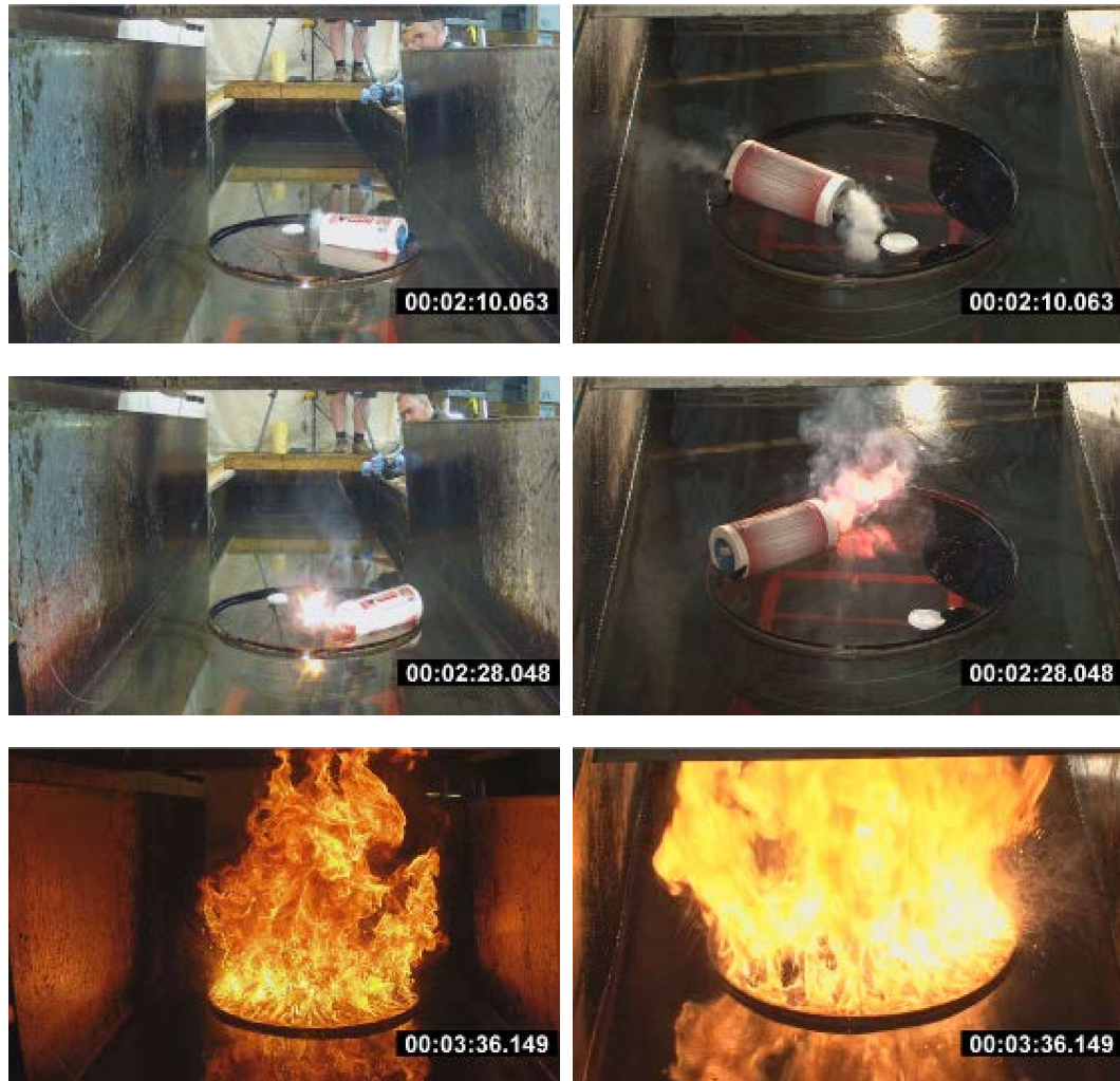
Figure 68. Test #12 Successful burn with Jet A1
