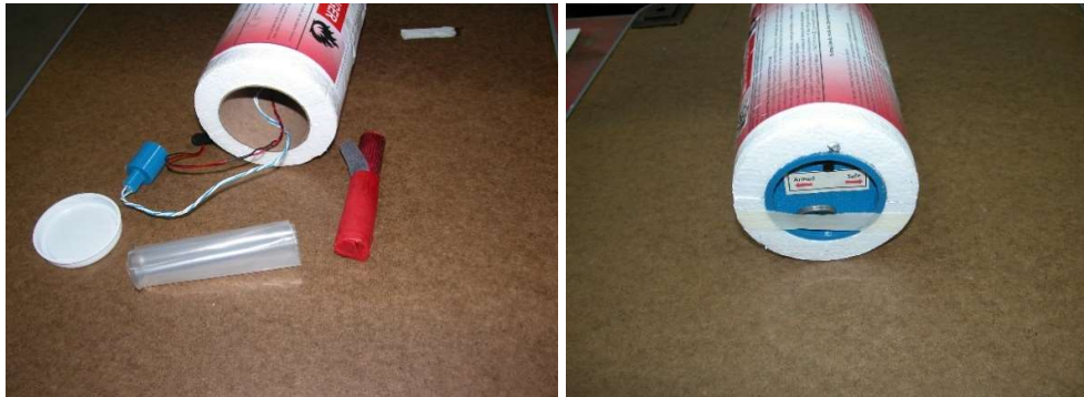
Figure 6. Igniter Details of end cap and contents. (Control end left – Igniter end right)
