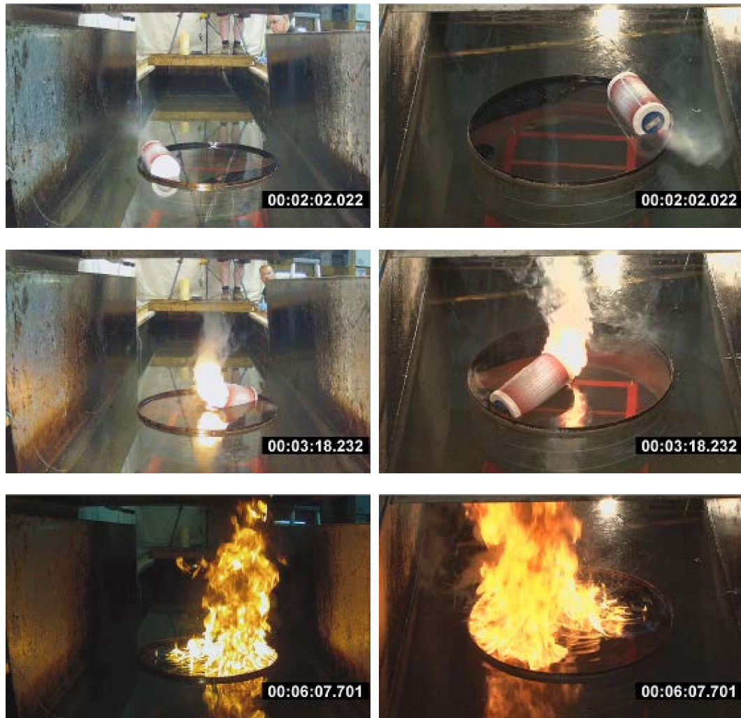
Figure 69. Test #13 Successful burn with premium gas
