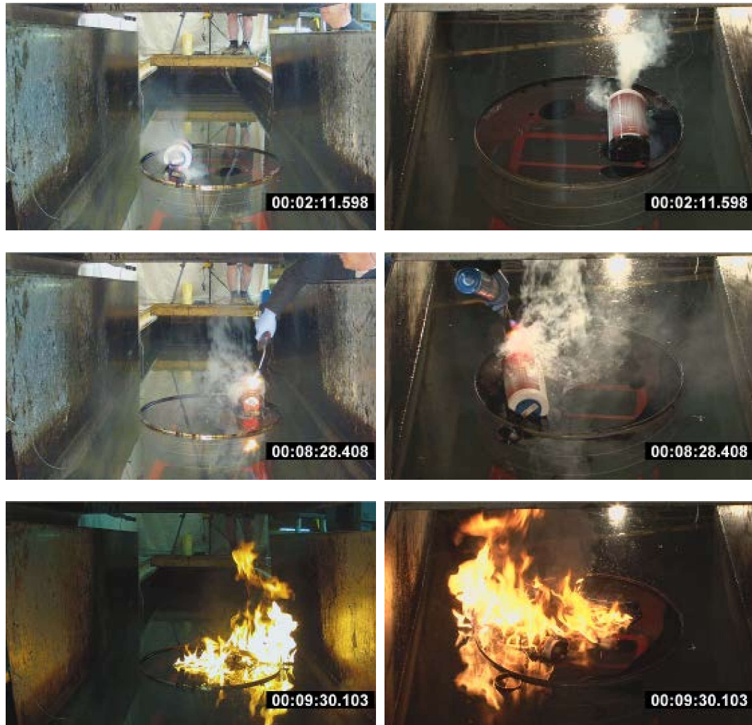
Figure 66. Test #10 Unsuccessful igniter test: crude lit with propane torch
