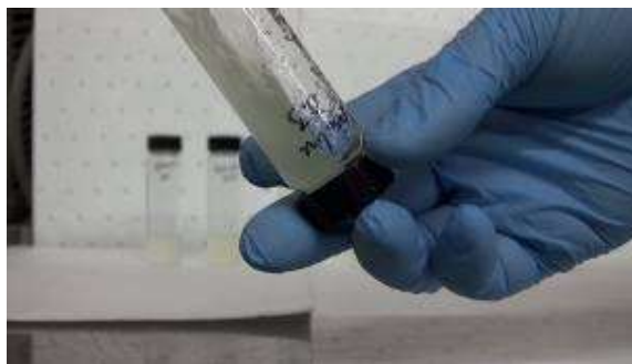
Figure 13. 15°C Gasoline at 5 minutes with 0.30g gel
