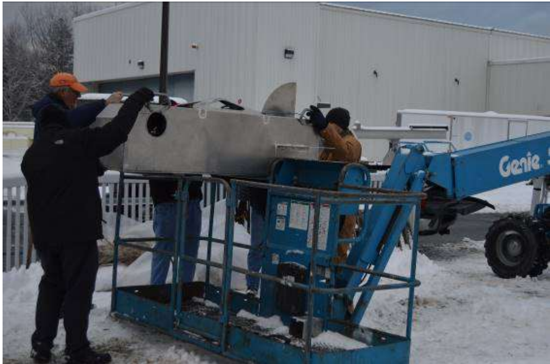
Figure 80 Loading IIHAS on to person lift for pre-test (note access port cut into side)
