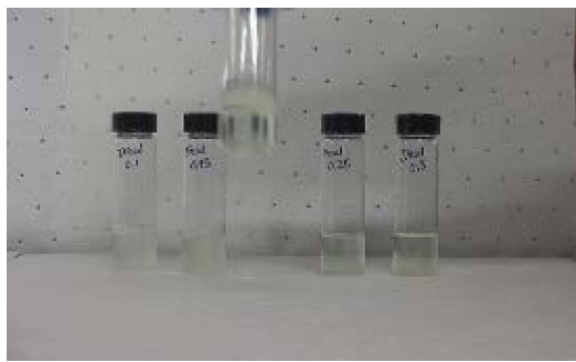
Figure 41. 15°C Diesel at 30 minutes with 0.20g gel
