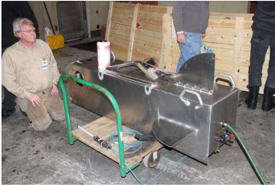
Figure 71 Integrated Igniter/Herder Application System with cover on
