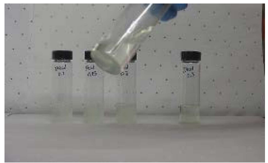
Figure 42. 15°C Diesel at 30 minutes with 0.25g gel
