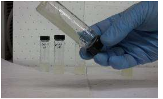
Figure 17. 15°C Gasoline at 20 minutes with 0.25g gel
