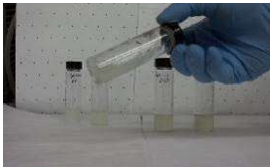
Figure 21. 15°C Gasoline at 30 minutes with 0.20g gel
