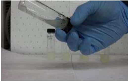
Figure 14. 15°C Gasoline at 20 minutes with 0.10g gel
