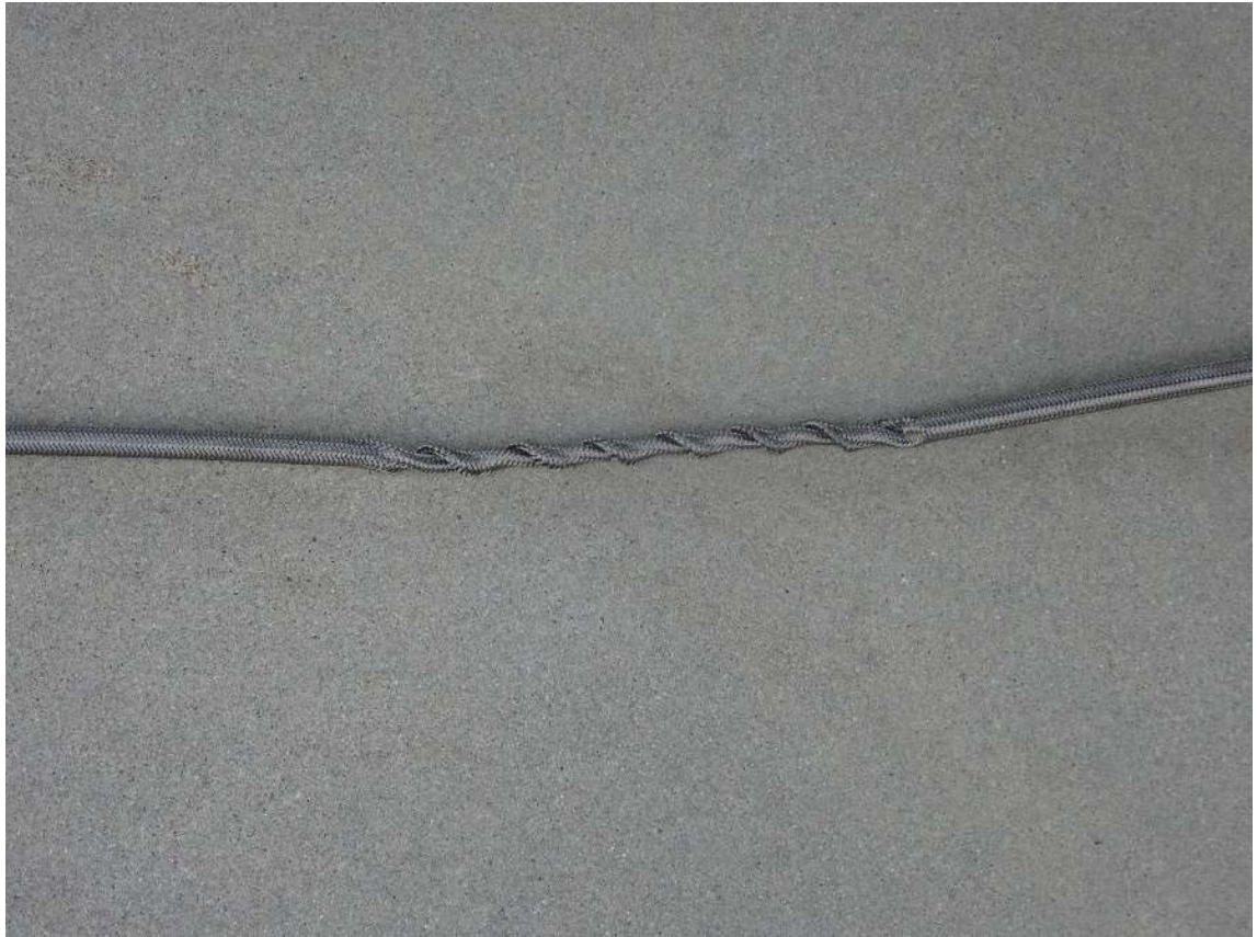
Figure 8770. Braided steel hose twisted during flight tests.
