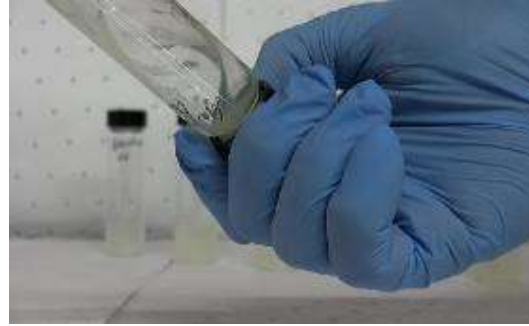
Figure 27. 15°C Gasoline at 60 minutes with 0.25g gel
