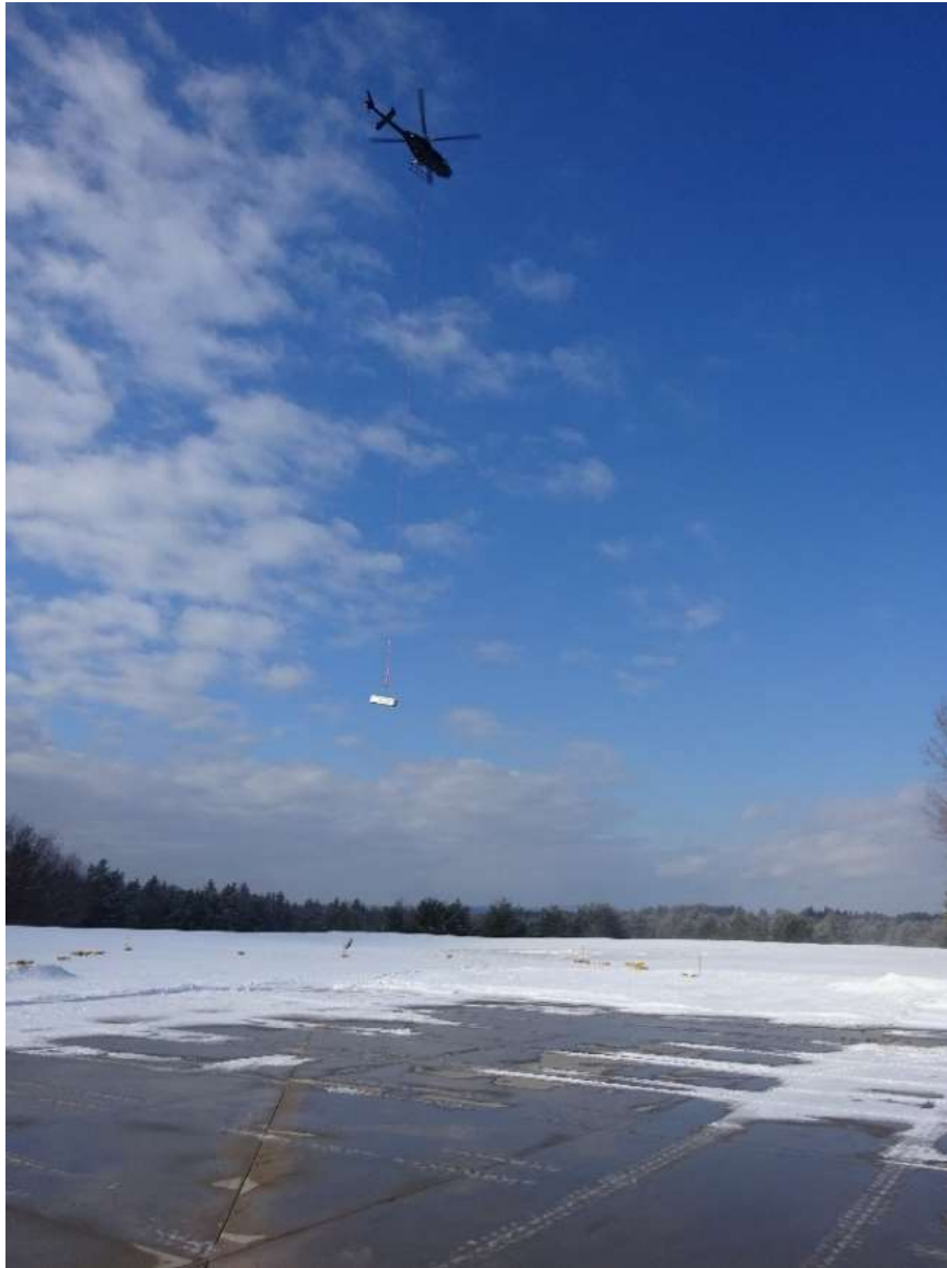
Figure 86. SIM in flight in original horizontal configuration.
