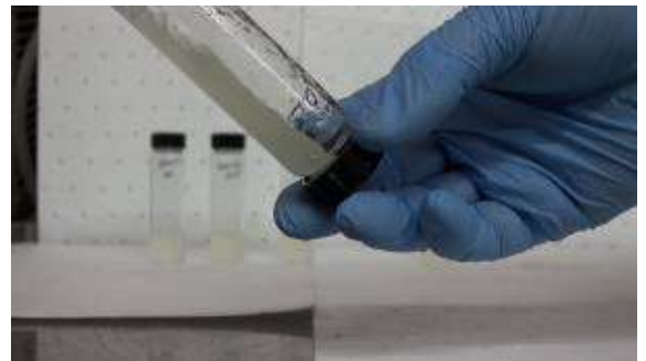
Figure 12. 15°C Gasoline at 5 minutes with 0.25g gel
