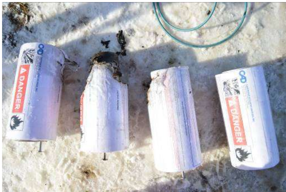
Figure 84 Igniter damage after Test 1 misfire (second from left went off)
