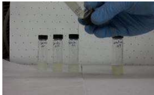
Figure 22. 15°C Gasoline at 30 minutes with 0.25g gel
