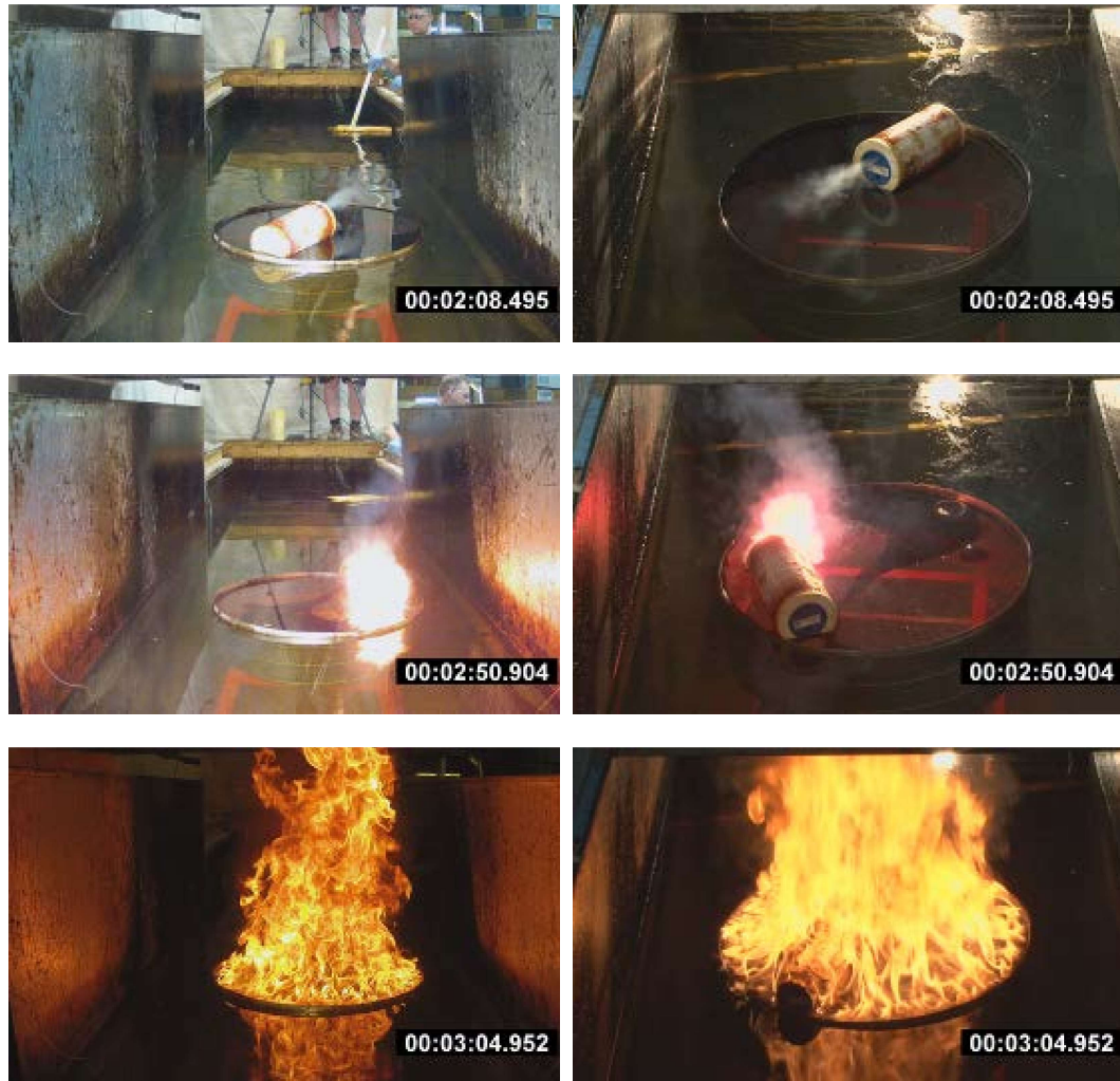
Figure 64. Test #8 Successful burn with premium gasoline
