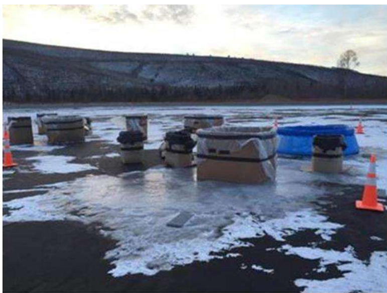
Figure E-7: Iceberg Form Tests Using Boxes and Inflatable Pool
