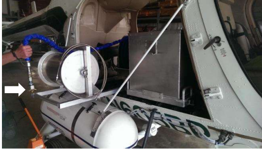
Figure 30: Herder Application System: Nozzle Assembly
