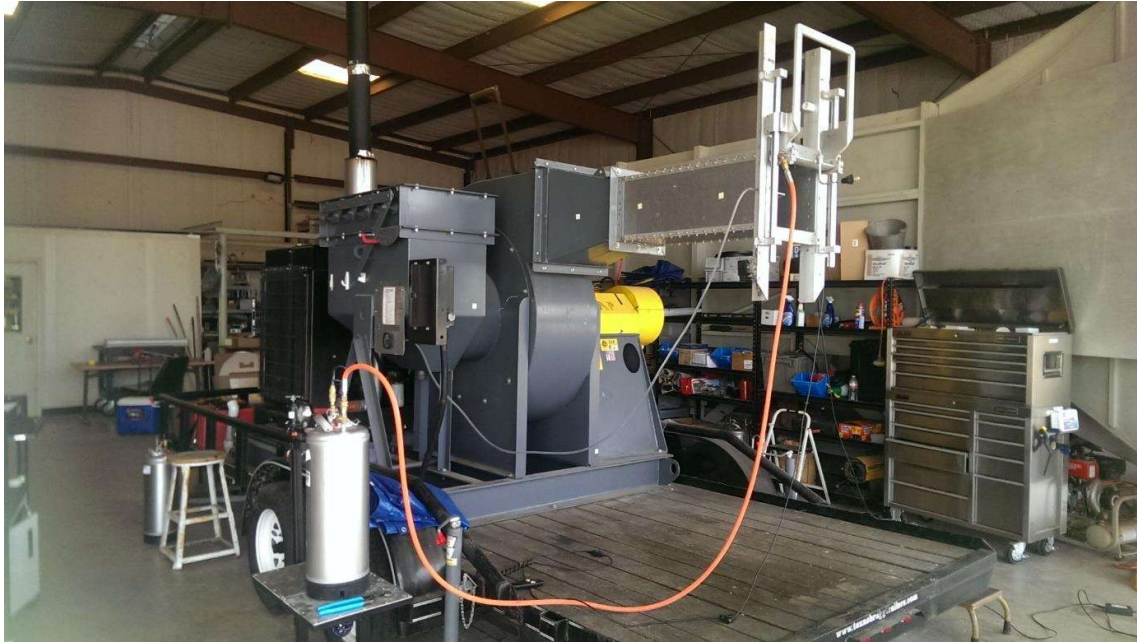
Figure 24: Wind Tunnel for Nozzle Testing
