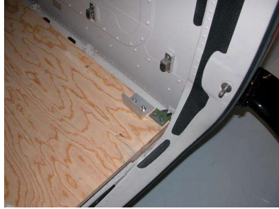
Figure 37: Rear seat belt attachment brackets
