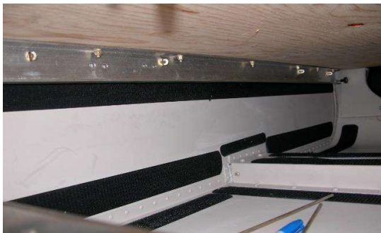
Figure 38: Forward seat belt attach points with machined stiffener bracket
