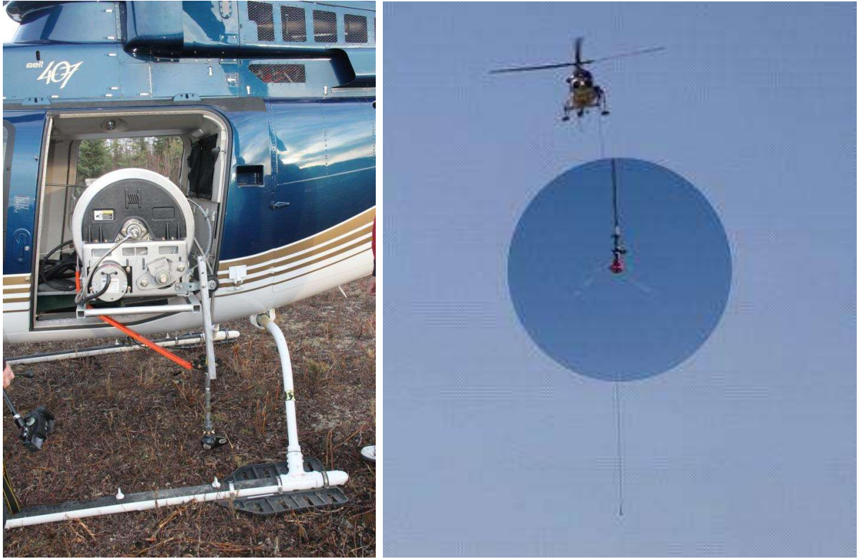
Figure ES-2: Herder application system mounted in Bell 407 and operating over basin
