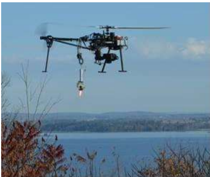
Figure 77: Responder triggering modified flare ignition
