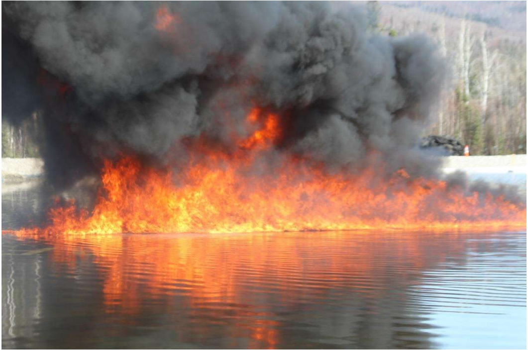
Figure ES-5: Successful burn of free-floating ANS crude oil slick herded with TS 6535 in Test 5
