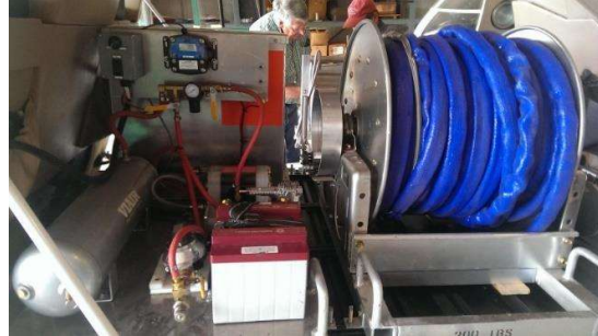
Figure 31: Herder Application System: Controls and Reel
