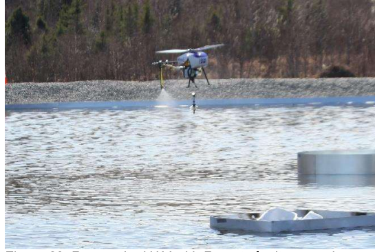
Figure 63: Responder UAV with Remote Igniter spraying simulated herder
