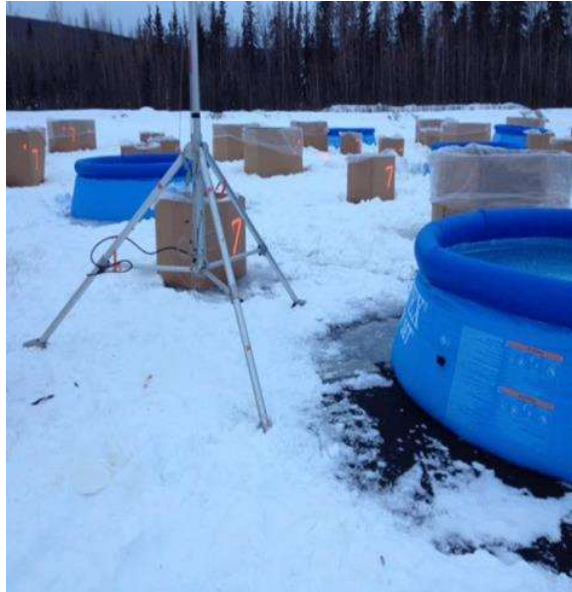
Figure B-14: Thermocouples and Data Logger locations within the Test Basin Centroid
