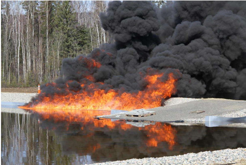
Figure 56: Burn against ramp and northeast sidewall of basin (Test 4)
