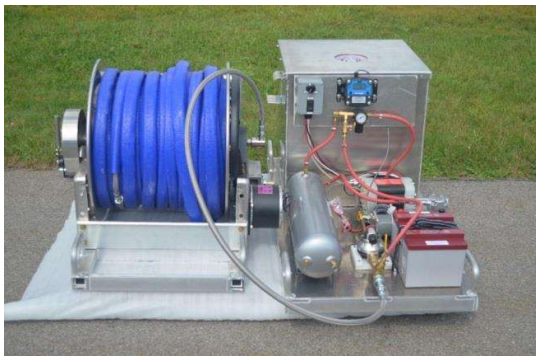
Figure 22: Initial Prototype Herder Application System Front
