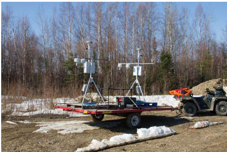
Figure 16: Trailer-mounted air samplers
