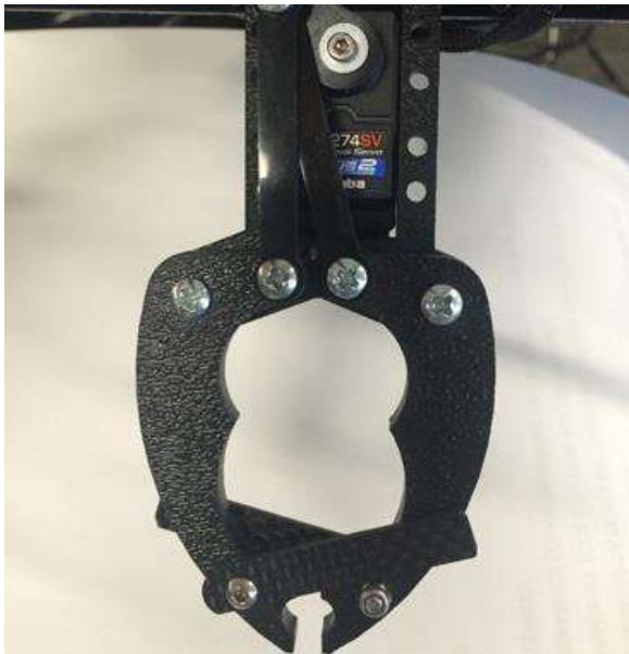
Figure 68: Retaining claw with redesigned retention bars
