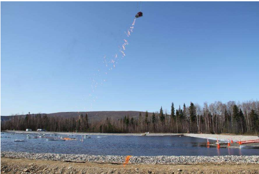
Figure 47: Successful Heli-torch test with 85:15 mixture of gasoline and diesel and longer gelling time
