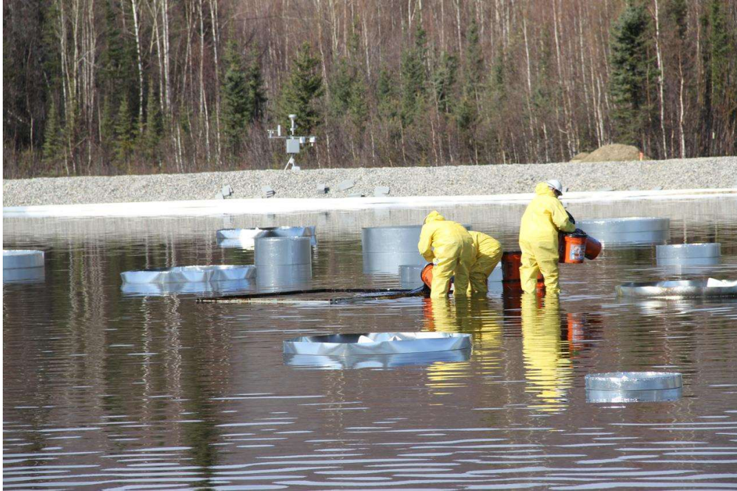
Figure 12: Pouring pre-weighed buckets of ANS crude into release frame in centre of "faux" floe field
