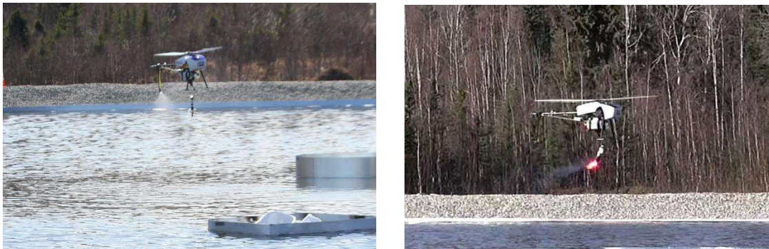
Figure ES-6: Responder UAV spraying simulated herder and carrying ignited flare
