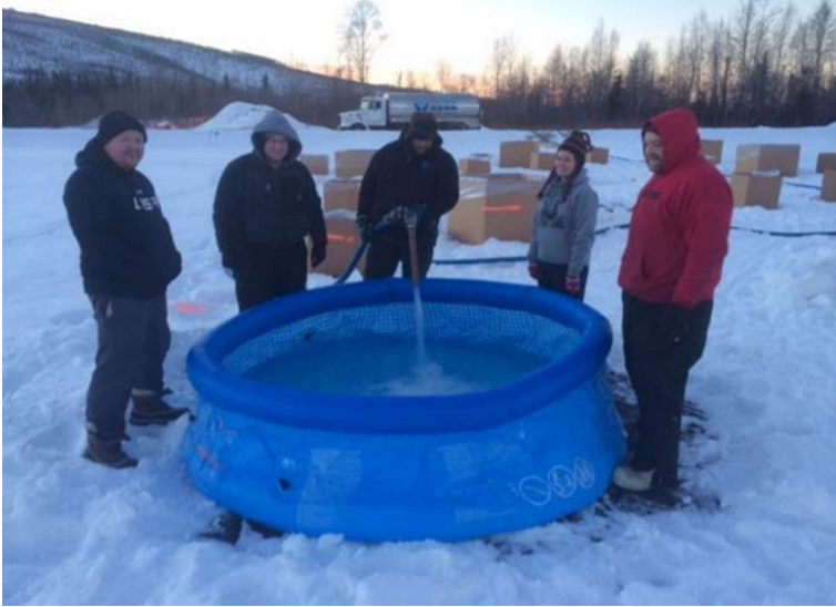
Figure B-10: Filling of 8 foot diameter pool for iceberg development from water truck
