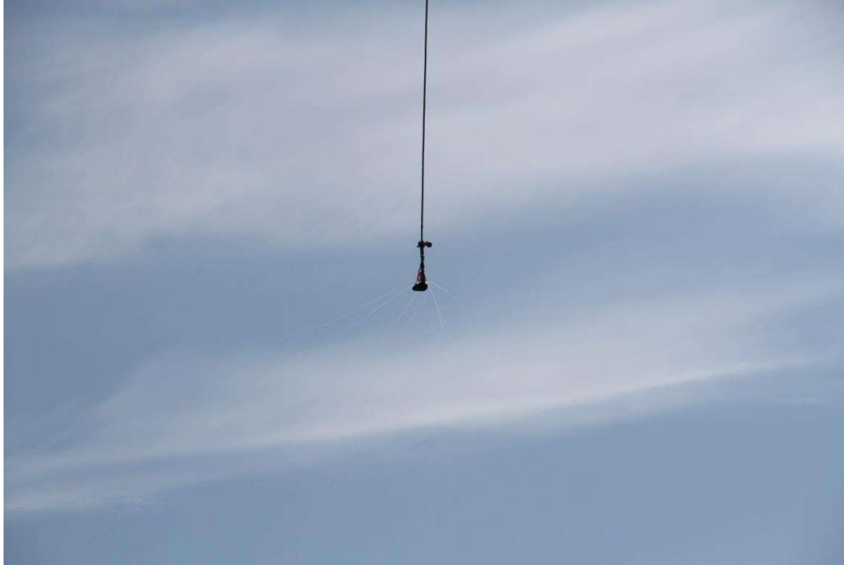
Figure 54: Herder streaming from nozzle when air pressure used to purge system at end of Run 4
