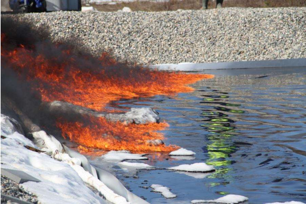
Figure 46: Test 2 burn in corner of basin
