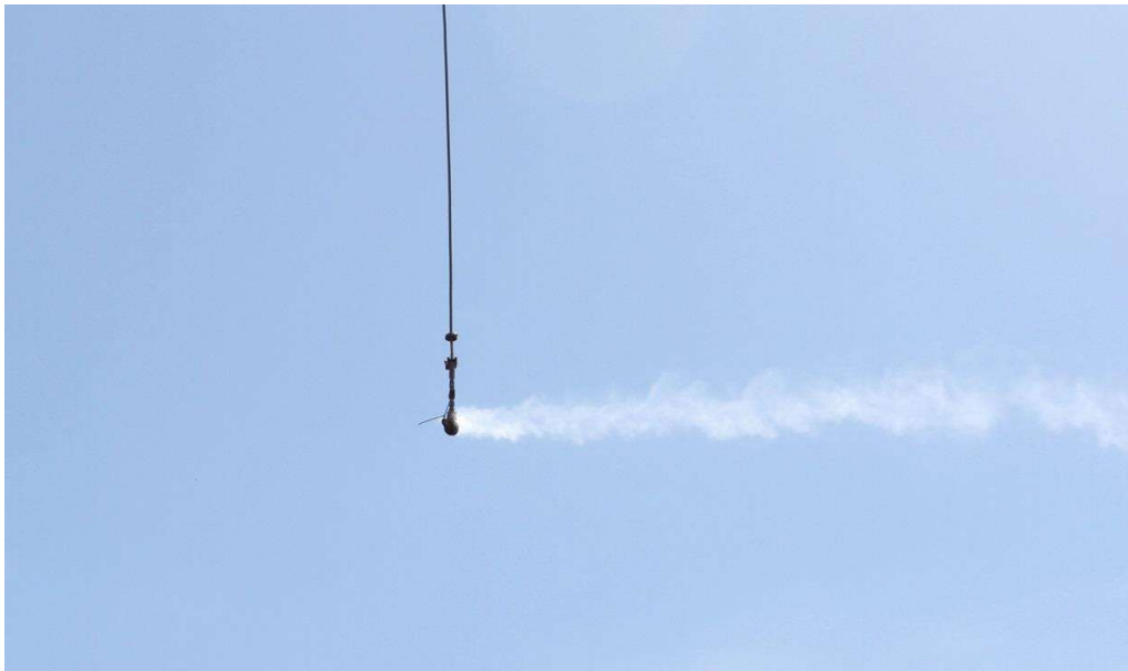
Figure 57: Good atomization of TS 6535 during Test 5 application
