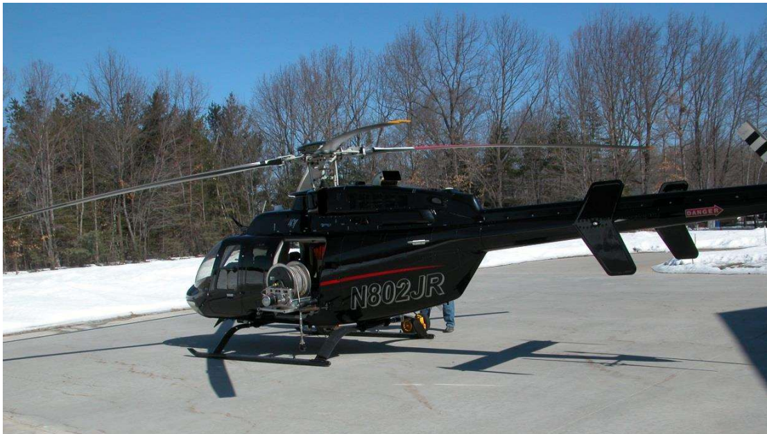
Figure 35: System installed in Bell 407 helicopter
