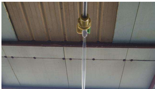
Figure 28: CP Products 2008 Nozzle with ThickSlick 6535
