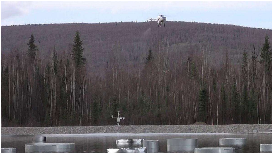
Figure 61: Responder UAV spraying water to simulate herder application
