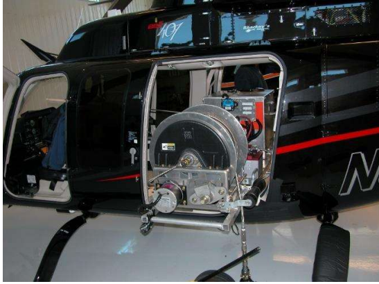
Figure 36: Hose reel extended out from helicopter
