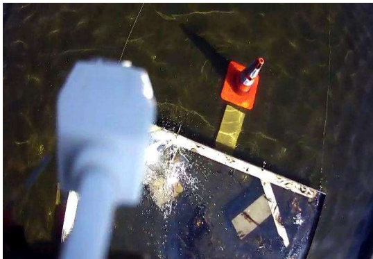
Figure 66: UAV Responder on-board view of successful flare release
