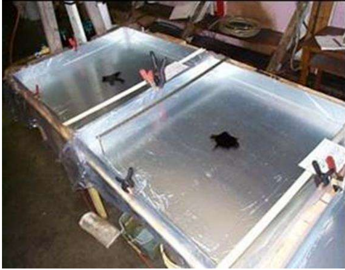
Figure F-1: Lined 1-m 2 Steel Pans Used For Experiments
