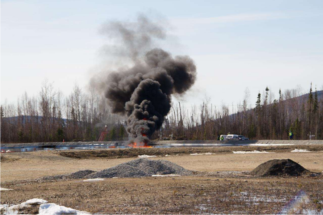
Figure ES-4: Successful burn of free-floating ANS crude oil slick herded with OP-40 in Test 3
