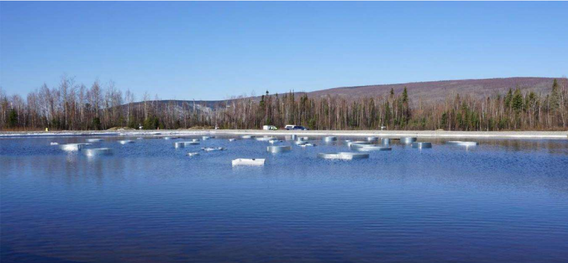
Figure B-17: Basin with "faux" bergs, sorbent, and oil release mechanism – prepared for test initiation
