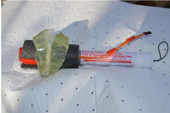
Figure 67: Marine Flare based Igniter System
