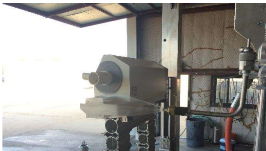
Figure 27: Flat Fan 8008 Nozzle with ThickSlick
