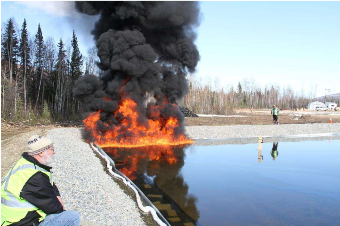
Figure 43: Crude burning in NW corner of basin (Test 1)
