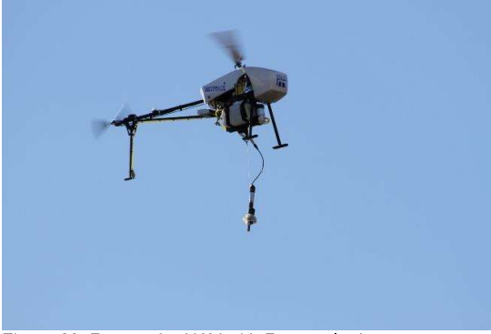
Figure 62: Responder UAV with Remote Igniter
