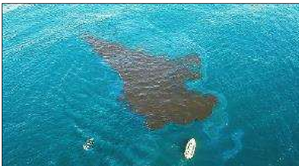
Figure 8.13 HISB 4.2 slick with compact area of thick oil surrounded by sheen.
