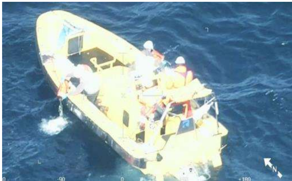
Figure 8.31 Herder poured on to the sea surface (Finnish Border Guard / SYKE)
