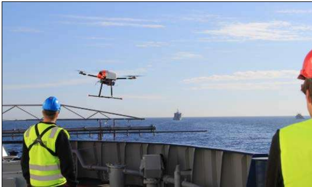
Figure 8.36 Take-off from MS Strilborg for sampling drone with SidePak and sampling train for sampling of soot, PAH's and BTEX's in the smoke plume
