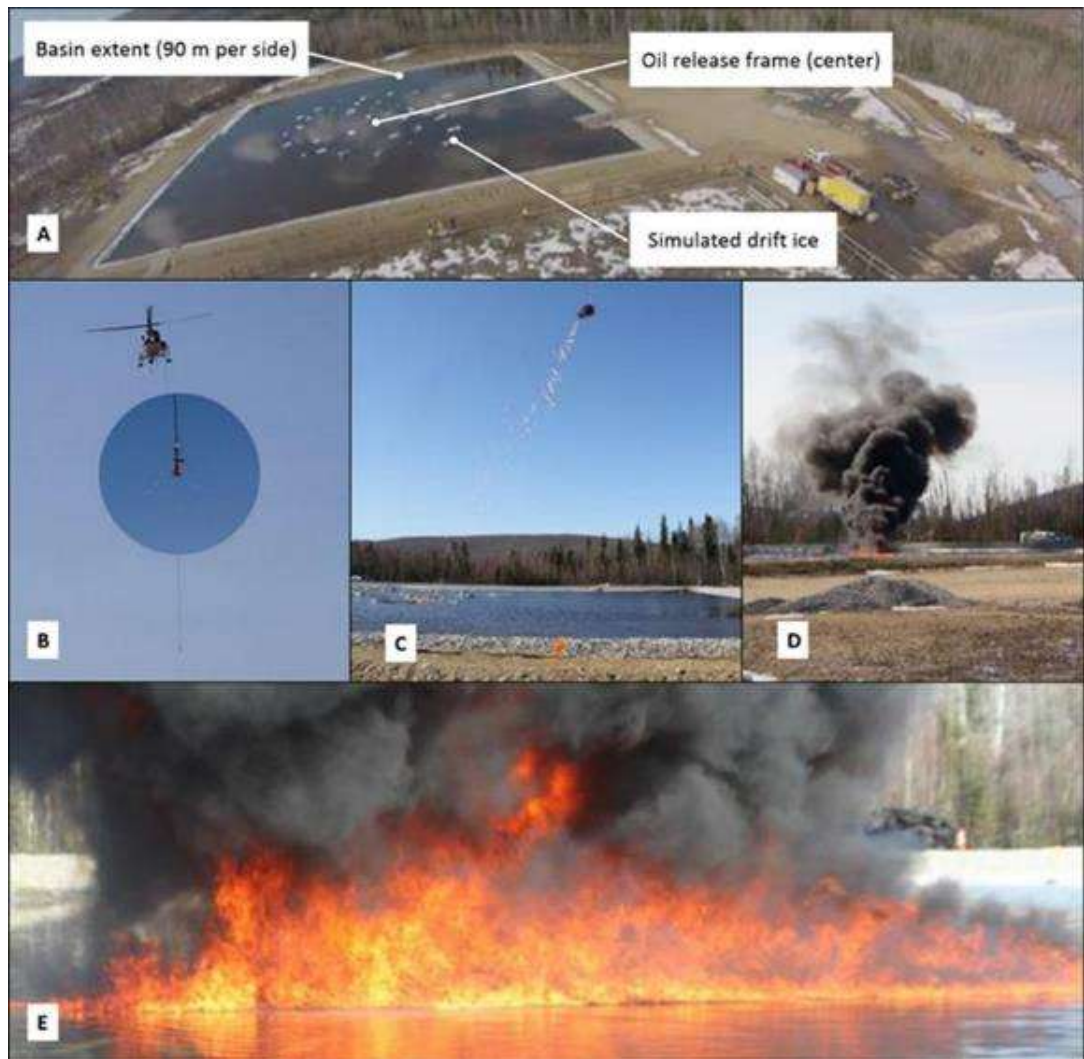
Figure 2.1 Field Test of Helicopter Herder Application and Crude Oil Ignition.
