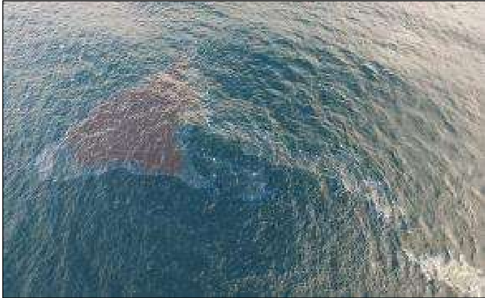
Figure 8.22 HISB 4.3 slick starting to spread out 4 minutes after oil release ended
