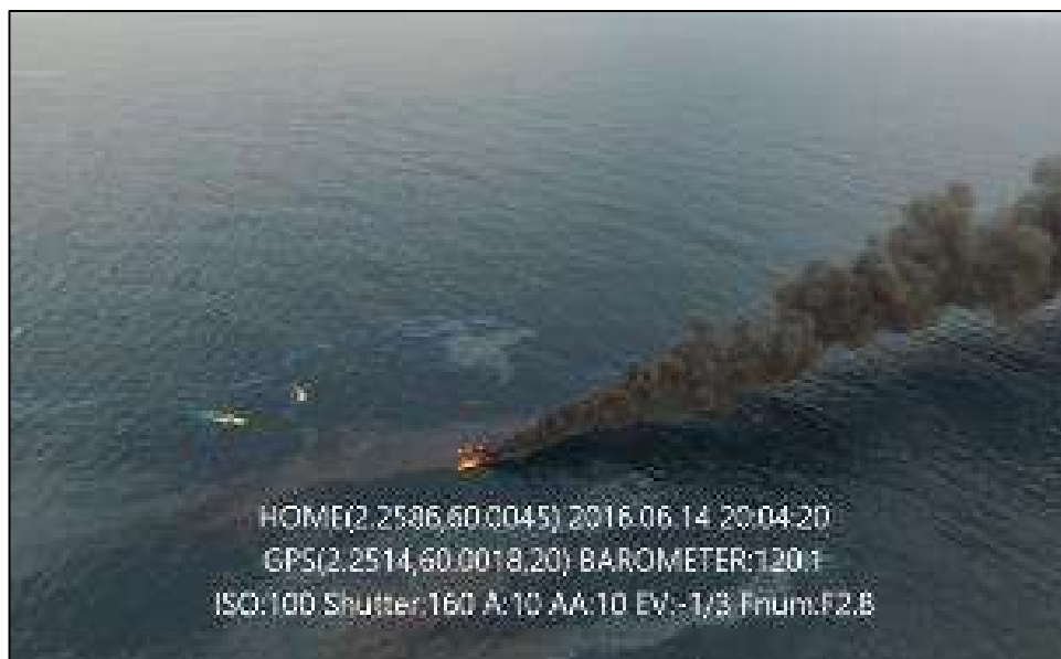
Figure 8.29 Second burn fully developed in HISB 4.3 (A) and extinguished after eight minutes (B).
