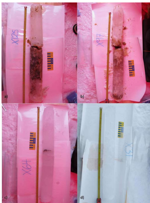
Figure 15 Example of cores collected at T3: a) Crude oil treatment, b) Oil+dispersant treatment, c) Burnt oil treatment and d) Control treatment
