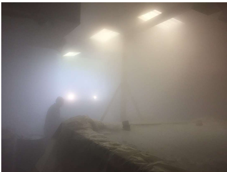
Figure 6 Condensation in the lab as the temperature warmed to outside air temperature while the bay doors were open.
