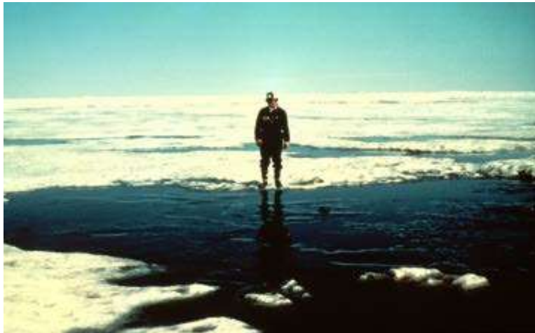
Figure 11. Oil blown to downwind edge of melt pools as 1-cm thick slicks (Source: Dome Petroleum).
