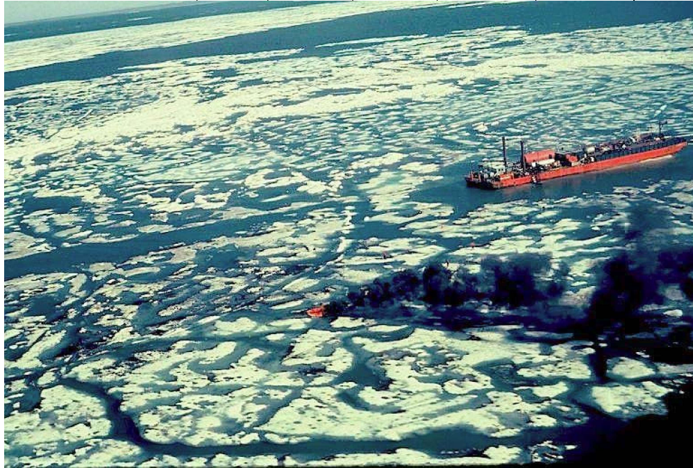
Figure 15. Burning oil on melt pools with igniters dropped from a helicopter during a simulated blowout under ice in McKinley Bay NWT (Source: Dome Petroleum).
