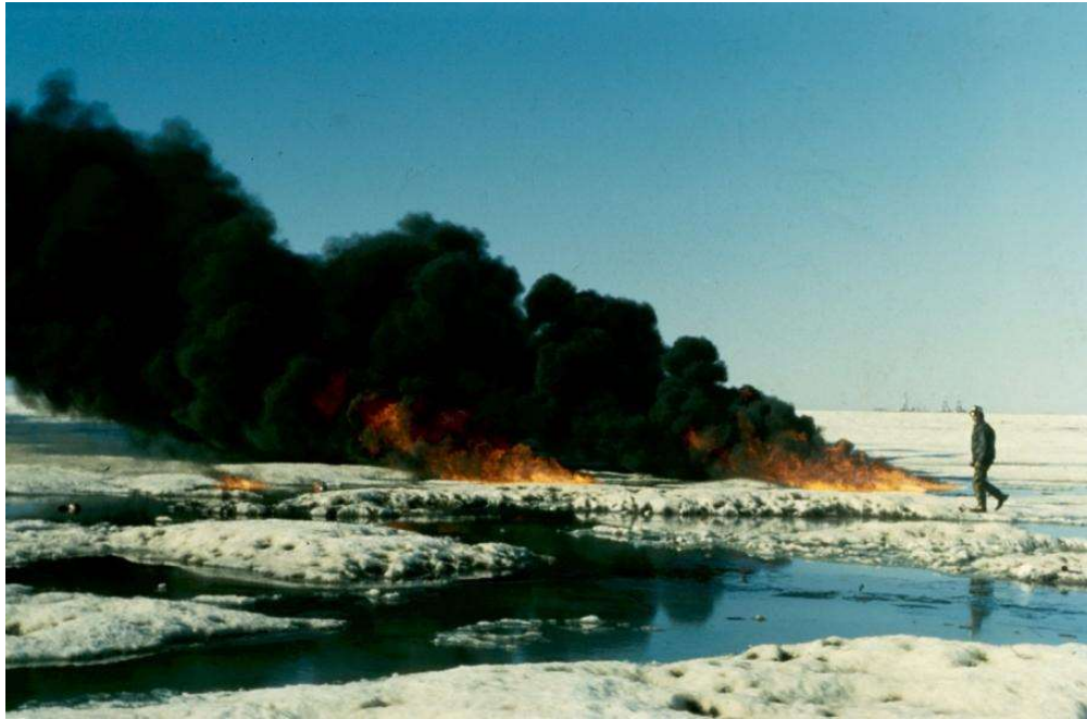
Figure 16. Ignition and burning of oil on melt pools is effective removal technique, with efficiency depending on oil distribution and igniter targeting (Source: Dome Petroleum).
